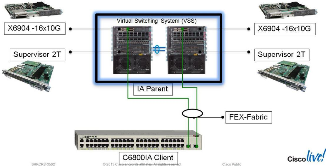
The Cisco Cat 3560CX-12PD-S or Cisco Cat 3560CX-8XPD-S can replace the C6800IA client in the configuration depicted in the figure above. The list of line cards that are supported on the IA Parent switch in the IA Parent-Child connection is restricted to – WS-X6904-40G, C6800-32P10G-XL, C6800-16P10G-XL and C6800-8P10G-XL.
