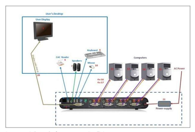
Figure 2 – Typical example of 4-Port KVM TOE installation
