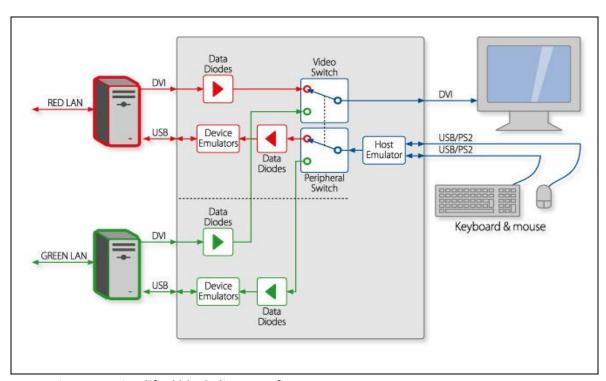
Figure 7 – Simplified block diagram of 2-Port KVM TOE
