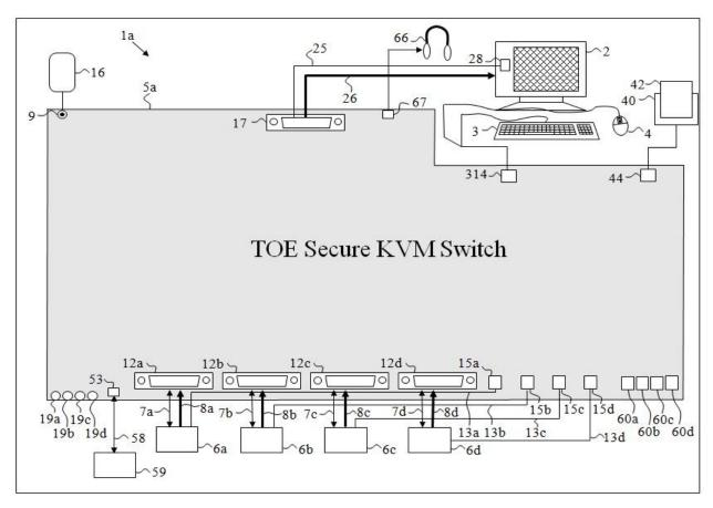
Figure 3 - Secure KVM Switch TOE external interfaces diagram
