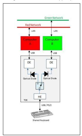
Figure 1 - TOE simplified block-diagram
