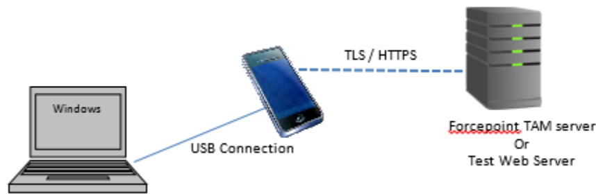
Figure 1: Forcepoint TAM Client TOE Test Environment Setup
