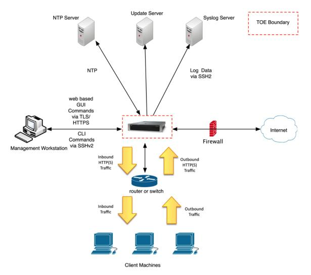
Figure 1 TOE Example Deployment
