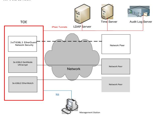
All devices operate in the same operational environment. IPsec tunnels are used to secure the communication between the device and external servers such as NTP server, Audit log server and LDAP server. All devices offer the same HTTPS/TLS based GUI interface for device configuration and management.
