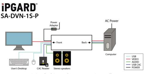
Figure 1: Standard Setup of 1-Port KVM TOE Installation
