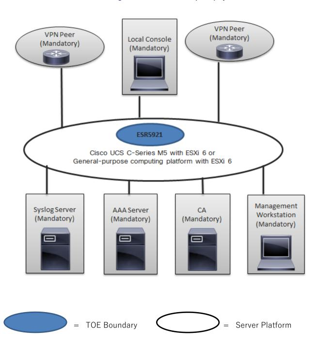
Figure 1 ESR 5921 TOE Example Deployment
