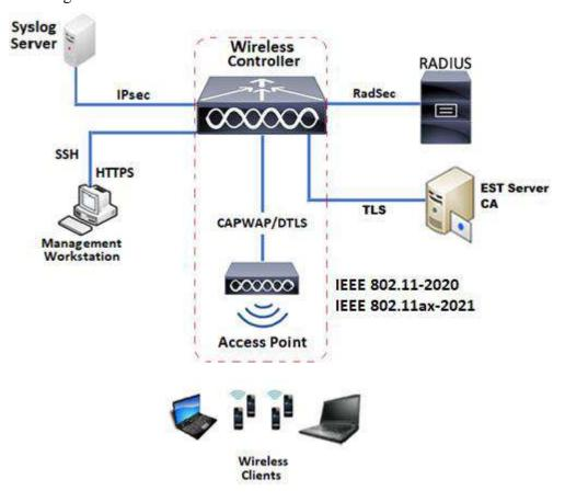
The WLC can be administered interactively using a local console connection (CLI), or remotely over HTTPS (GUI) or SSH (CLI). Once the APs have registered with a Controller and 'joined' to form the TOE, the APs are entirely managed via the WLC. The TOE does not permit direct local administration of the APs thus fulfilling distributed TOE use case 1 in section 3.1 of [NDcPP].
