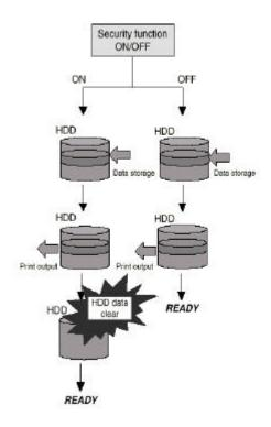
Figure 11. DSK HDD-Erase Security Function
