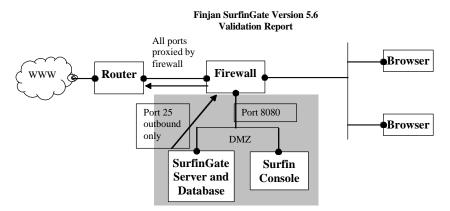
Figure 2: SurfinGate Evaluated Configuration
