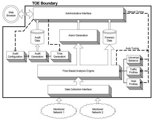
Figure 1 StealthWatch Component Architecture
