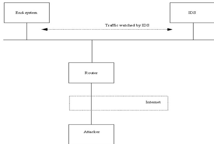
**Figure 1: Example Network Topology Using an IDSM2**
