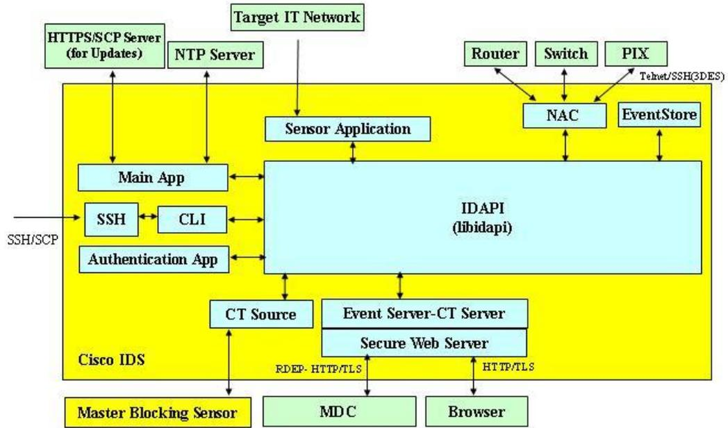
Figure 4: Logical Components of the TOE
