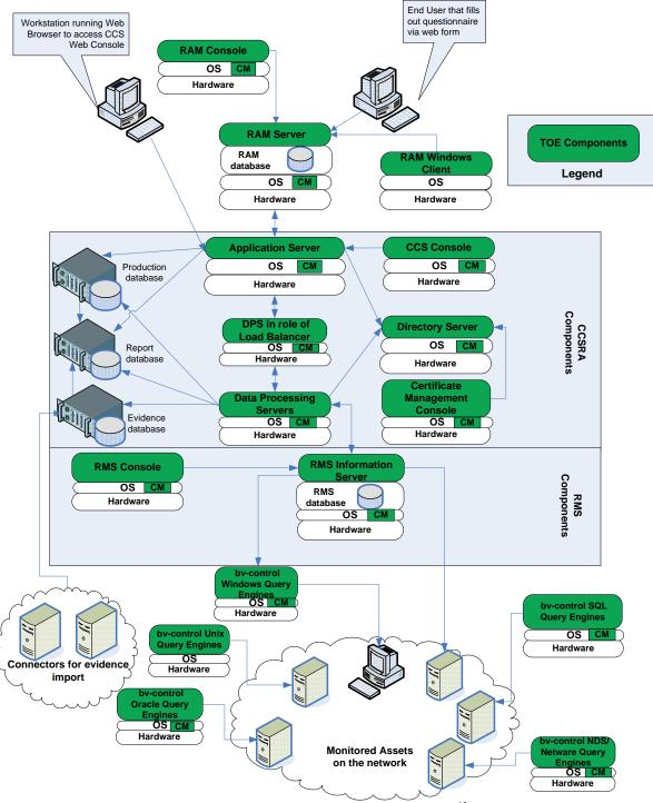
Figure I - Sample Deployment of the TOE<sup>12</sup>
