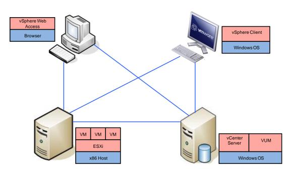
Figure I - Evaluated Deployment Configuration of the TOE
